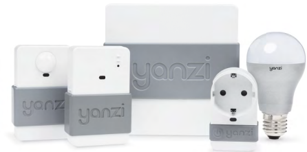
Fig. 1. Yanzi Networks system. The nodes use a STM32W108 system-on-chip and run the Contiki OS.
