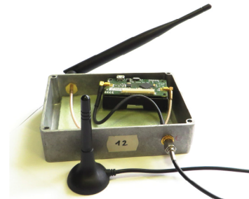
Fig. 5. A measurement device with dual-radios used in the demonstration
